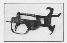
ABOVE: Right side of Type 63 trigger mechanism, showing the selector lever.
